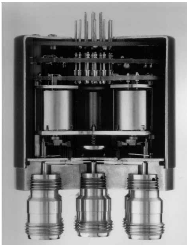
Figure 2: a cutaway view of RAMSES coaxial switch
